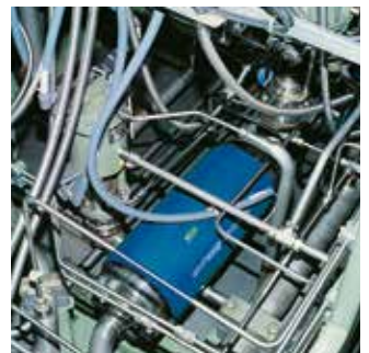
KRAL flowmeter installed in the engine room of a yacht.
