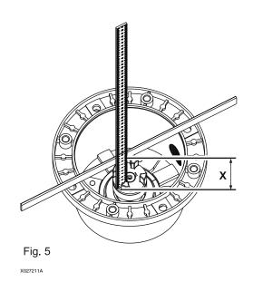
Mount the motor-side coupling half 052.2 on the shaft end of the motor, see Fig.
