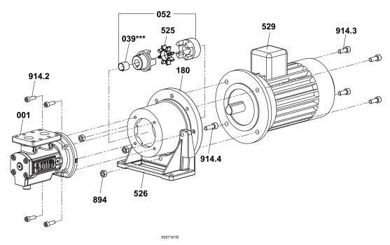
Fig. 2.Completion elastomer coupling ALP 15-85
