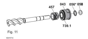
6. Remove the remaining parts of the mechanical seal 457 from the main screw, see Fig. 11.
