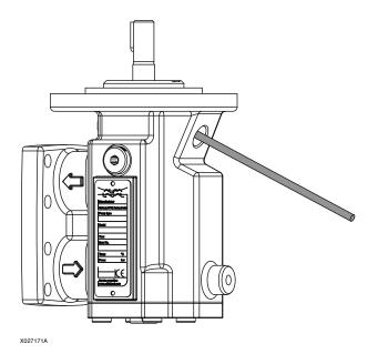
Fig. 1 Cleaning the leakage vent hole
